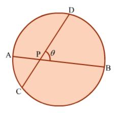
• If two chords of a circle intersect such that one chord has sub-segment lengths *a* and *b* and the other has sub-segment lengths *c* and *d*, then *ab* = *cd*.
